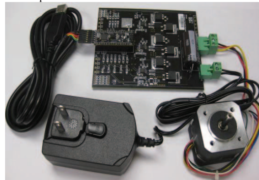
Fig.5 Configurable 3-phase PMSM with a USB-UART bridge and universal power adapte
